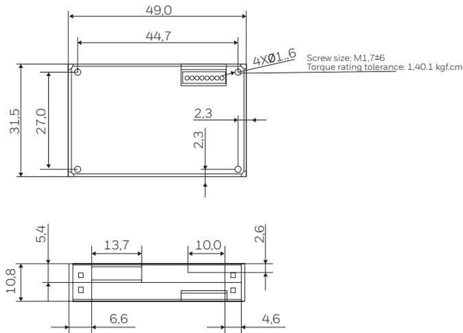
Figure 6b. IH-PMC-002 (Air in-and-out on opposite sides)
